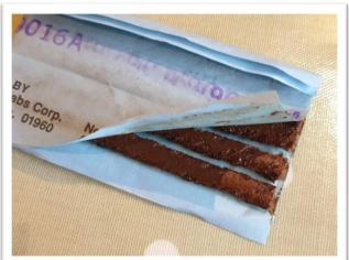
The plugs look like others I have seen and are TUV tested in Germany up to 186mph with a repair shear strength, up to 160kgs.
