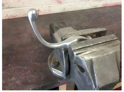
Gripping the lever in the vice, I applied the blow torch heat to where I wanted to bend the lever and used a piece of pipe to help with the bending. How much pressure on the pipe and how much heat was applied was anyone's guess. I figured that at some point with a bit of pressure on the pipe and enough heat, the lever would eventually move.
