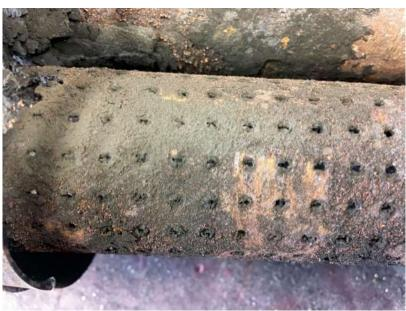
So I was left with the 2 end caps and a lot of mess. The mess went in the bin and I went on the interwebs to find exhaust part suppliers. I found a company that supplied 110mm internal diameter stainless tube, perforated stainless tube and exhaust wadding. Perfect.
