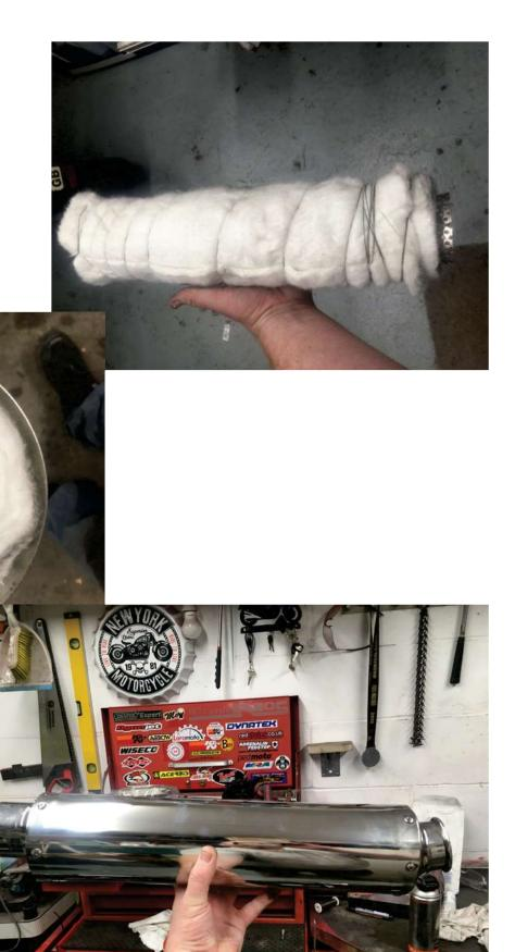
In the pictures you can see the perforated tube wrapped in the wadding, I slipped that inside the stainless tube and riveted it all together. I look forward to hearing how it sounds...
